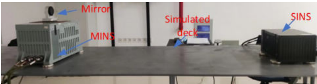
Fig. 4. Deformation measurement test environment
